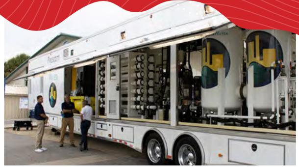
**Above:** Staff from Mote and Prescott Clean Water Technologies test how well the OZONIX® system can mitigate red tide.
